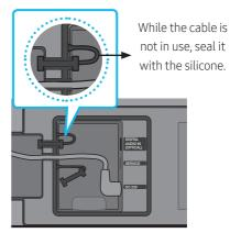
• After the cable is connected, close its cover and then tighten the loosened screws.
