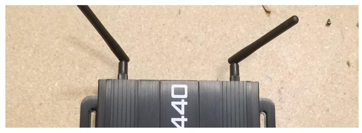
4. Secure the OS-440 onto the back aluminum mounting plate within the enclosure. This can be done using many methods. The method shown utilizes two of the predrilled and tapped holes (8-32) and one No. 8 self-drilling screw. **Note:** Before securing the OS-440 to the mounting plate, ensure that all wires/connectors can access the OS-440 without interfering with the enclosure.
