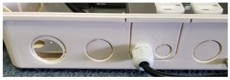
6. Insert rubber grommet into the knockout hole. A file or sand paper can be used to smooth out any rough edges. For a more water-tight seal, Altelix recommends using their HG series cable glands, see brochure inside original packaging.
