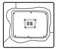
2. Locate termincal cup on the underside of the speaker.
