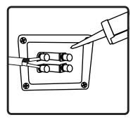
4. To seal the terminal cup for weatherproofing purposes, use a silicone gel and caulking gun. Be sure that wires are connected and speaker is functioning before sealing.
